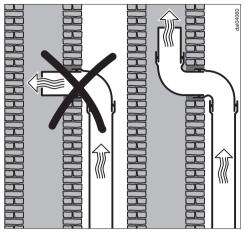
If the exhaust is ducted into an inactive flue, the air must be expelled parallel to the flow direction of the flue.
